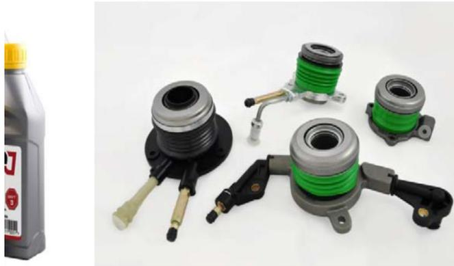
The concentric slave cylinder (CSC) is subjected to just as much natural wear as the clutch or flywheel and should be replaced every time the clutch is changed. There are a few important things to consider during installation in order to preserve the functionality and service life of the components.
