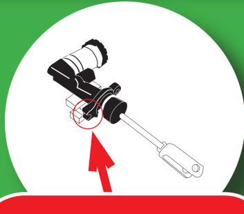
BROKEN MOUNTING BROKEN PUSHROD
