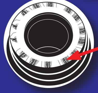
THE WEAR ON THE BEARING **CONTACT FACE INDICATES THIS ISSUE**
