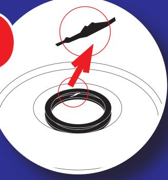
4) A CRACKED BODY **INDICATES INCORRECT** MOUNTING PROCEDURE OR **BLEEDING PROCEDURE -**NO RFC
